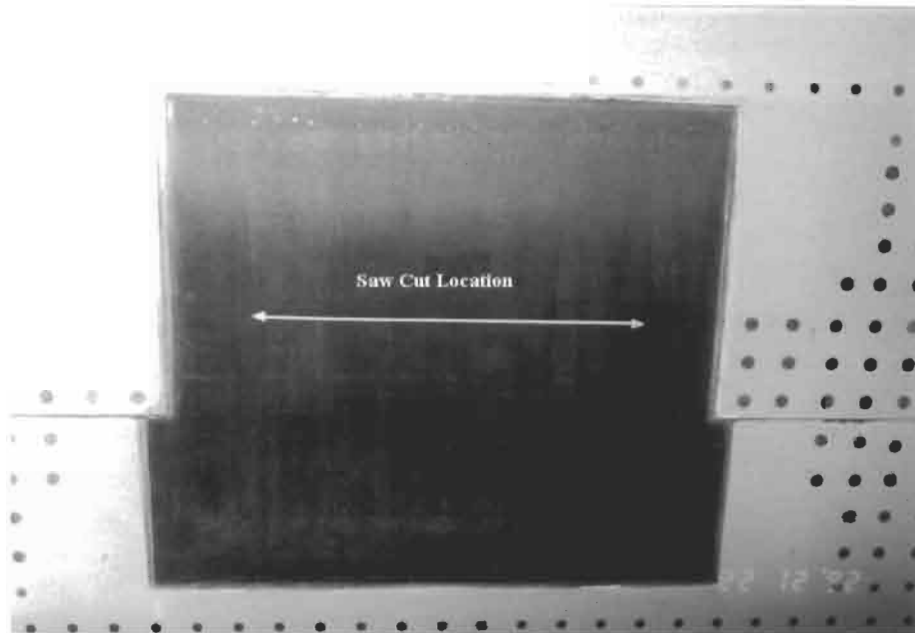
Fig. 16.24. Doubler installed on A330 lap joint.
