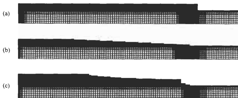
Fig. 10.4. Typical finite element meshes for three patch stepping cases: (a) single step case, (b) uniform stepping case, (c) non-uniform stepping case.
